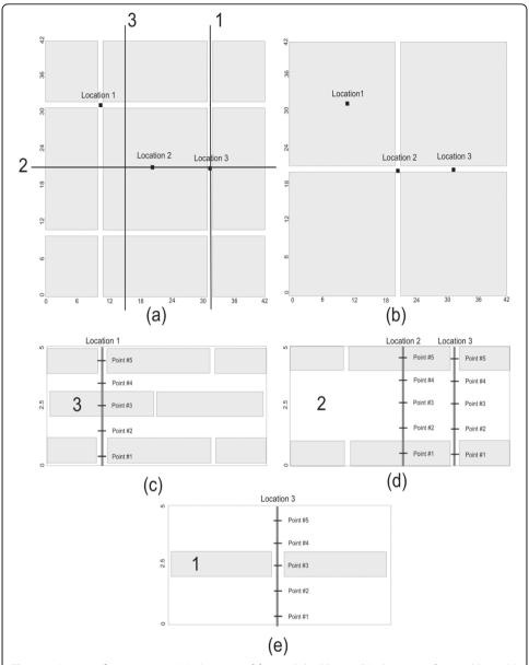
**Figure 4 Layers of corneocytes.** (a) plan view of first and third layers. (b) plan view of second layer. (c) (d) and (e) Cross-sections corresponding to lines 3, 2 and 1, respectively as indicated on (a). Location of concentration profiles and observation points for each depth indicated. Grid dimensions in metres for the scaled domain (5 m = 5  $\mu$ m).
