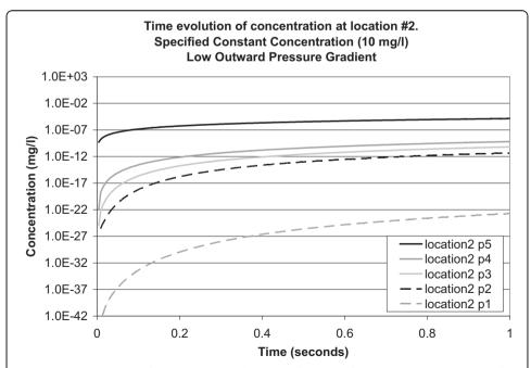
Figure 9 Time evolution of concentration at location 2 for a specified constant concentration of 10 mg/l applied to the top surface of the model (low outward pressure gradient). Concentration is plotted on a logarithmic scale. Location points are listed in the legend in their order of depth in the model (5 at the top and 1 at the bottom).
