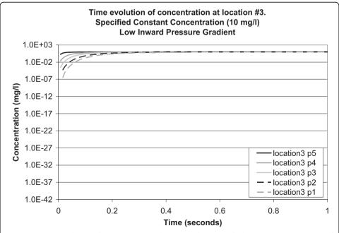
Figure 11 Time evolution of concentration at location 3 for a specified constant concentration of 10 mg/l applied to the top surface of the model (low inward pressure gradient). Concentration is plotted on a logarithmic scale. Location points are listed in the legend in their order of depth in the model (5 at the top and 1 at the bottom).
