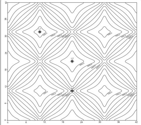
Figure 5 Plan view of head (pressure) contours within a 42  $\mu$ m  $\times$  42  $\mu$ m layer composed of intercellular channel lipids only, as obtained through MODFLOW simulation. Locations (L1, L2 and L3) of monitoring profiles shown.
