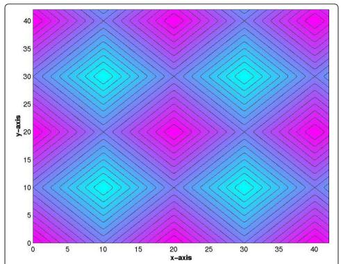
Figure 7 Analytic solution of pressure distribution within a 42  $\mu$ m  $\times$  42  $\mu$ m layer composed of intercellular channels, as obtained using Green's functions and the method of images.
