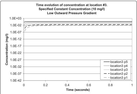
**Figure 8** Time evolution of concentration at location 3 for a specified constant concentration of 10 mg/l applied to the top surface of the model (low outward pressure gradient). Concentration is plotted on a logarithmic scale. Location points are listed in the legend in their order of depth in the model (5 at the top and 1 at the bottom).
