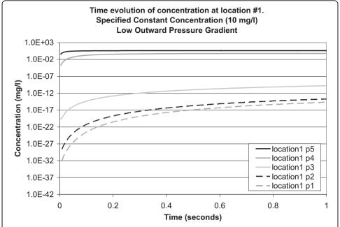
Figure 10 Time evolution of concentration at location 1 for a specified constant concentration of 10 mg/l applied to the top surface of the model (low outward pressure gradient). Concentration is plotted on a logarithmic scale. Location points are listed in the legend in their order of depth in the model (5 at the top and 1 at the bottom).
